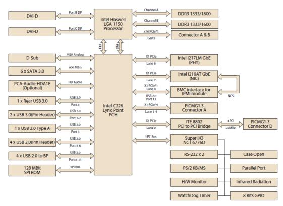
Figure 1.3 PCE-7128 block diagram
