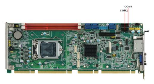
The PCE-5128/7128 offers two serial ports. These ports can connect to serial devices, such as a mouse or a printer, or to a communications network.
