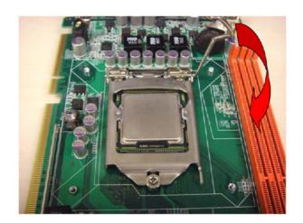
5. The finished processor installation.
