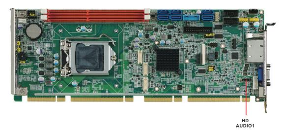
This HDAUD1 pin header is the connection interface to Advantech's 7.1 channel high definition audio module.
