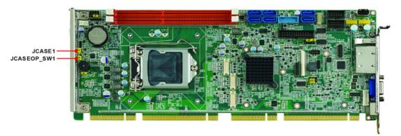
Figure 2.2 PCE-5128/7128 Case Open Jumper Locations
