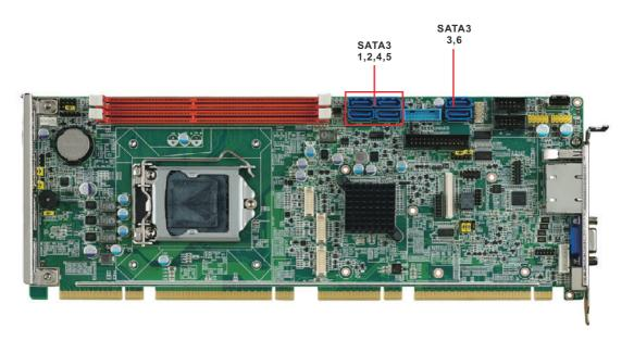
The PCE-5128/7128 features high performance serial ATA interface (2\* 600MB/s and 4\* 300MB/s) which eases cabling to hard drivers or CD/DVD drivers with long cables. These six on-board SATA ports can be configured as RAID 0, 1, 10, or 5. Please see the detailed BIOS setting instructions for this in Chapter 3.
