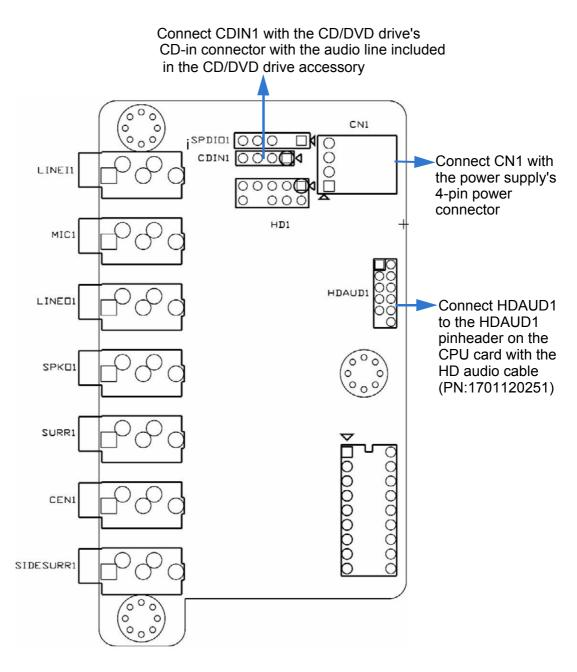
Figure 2.1 Jumper and connector locations of PCA-AUDIO-HDA1E
