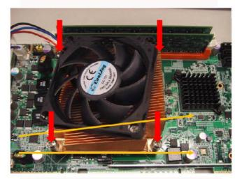
Note the direction of CPU cooler; it must follow that shown above. Installing a CPU cooler in the wrong direction may cause poor heat dissipation that may damage the CPU card.
