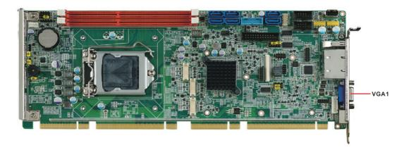
This CPU card has VGA outputs that can drive conventional CRT displays. VGA1 is a standard 15-pin D-SUB connector commonly used for VGA.
