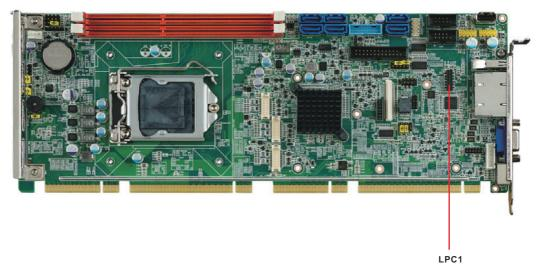
LPC1 is a 14-pin female pin header for connection with an Advantech LPC module.
