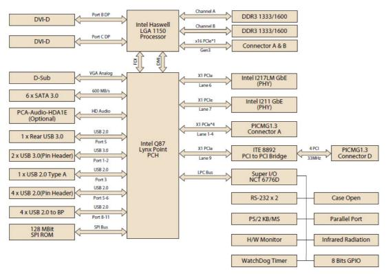
Figure 1.2 PCE-5128 block diagram
