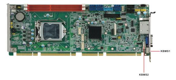
Two on-board 6-pin mini-DIN connectors (KBMS1) provide connection to a PS/2 keyboard and mouse by the Y-cable (1700060202) in the package.
