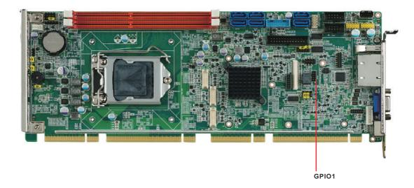
Provides 10-pin header connector for 8-bit Digital I/O usage. Refer to Appendix B for detailed information on the pin assignments and programming guide in Appendix C.
