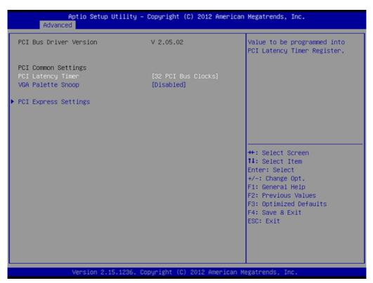
Figure 3.4 PCI Subsystem Settings
