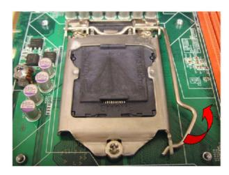
2. Remove the socket protection cap.
