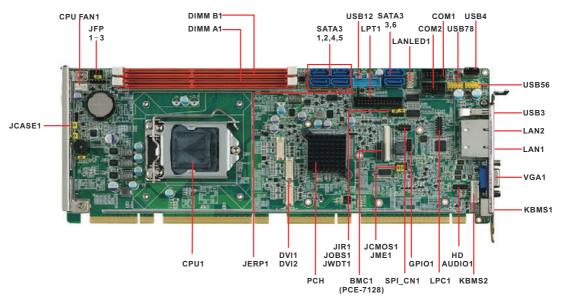
Figure 1.1 Jumper and connector locations
