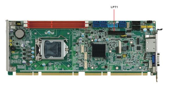
The parallel port is normally used to connect the motherboard to a printer. The PCE-5128/7128 includes an onboard parallel port, accessed through a 26-pin flat-cable connector, LPT1.
