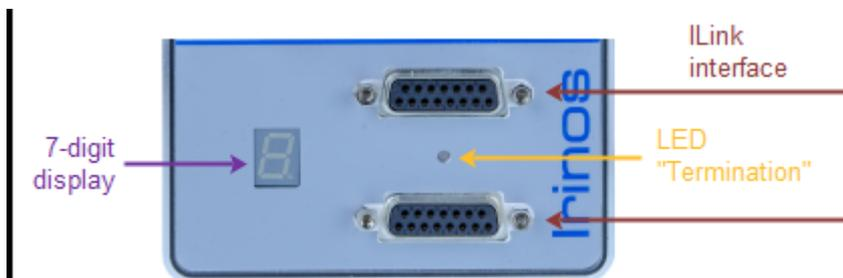
Connections and signalling elements of a "Slave-Box"
