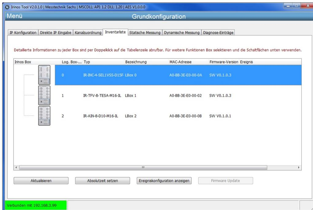
Changes can be obtained by pressing the "Update" button. However, any modification to the system setup, such as adding or removing boxes, requires a power-off-power-on cycle at the master box before it can be detected by the Irinos Tool.
