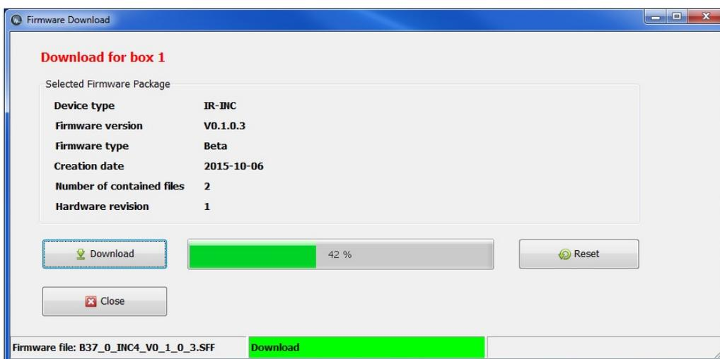
After all packages have been downloaded to the Irinos system, a system reset is required to activate the downloaded firmware. Pressing the "Reset" button sends an appropriate command to the Irinos system.
