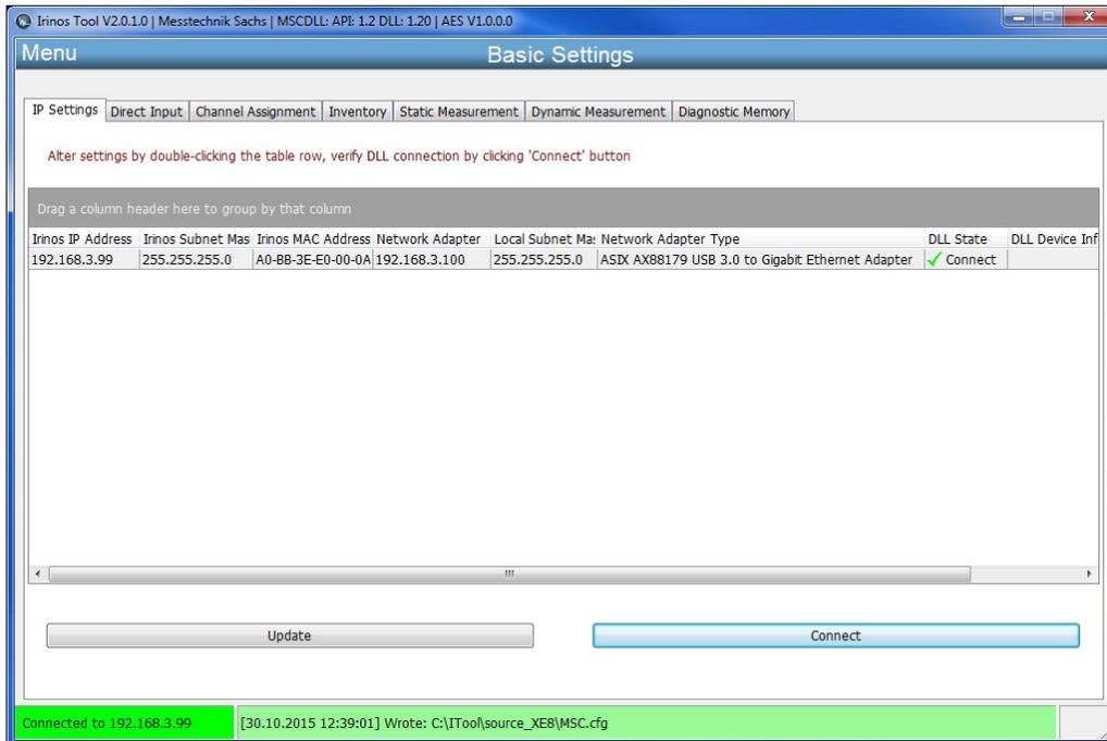
If the connection check fails, the "DLL State" column is showing a red error sign followed by the error reason, as delivered by the DLL while trying to access the box. The connection status at the bottom status bar indicates "Not connected".
