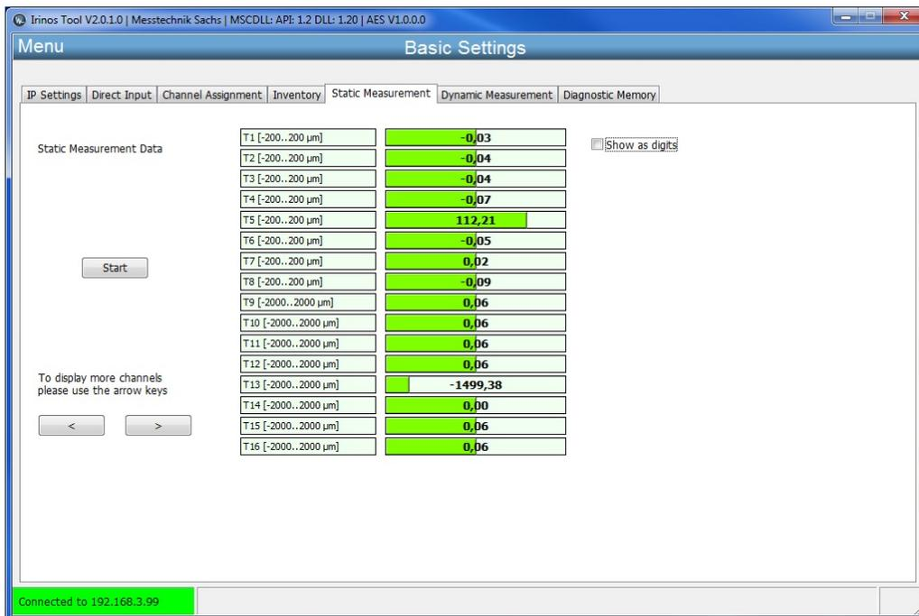
Static measurement is automatically set-up by [verifying the connection](#)<sup>[37]</sup>, as it is used as a timeout-monitoring function. Whenever the user directly enters the Static Measurement window, it might be necessary to start the static measurement by means of the "Start" button.
