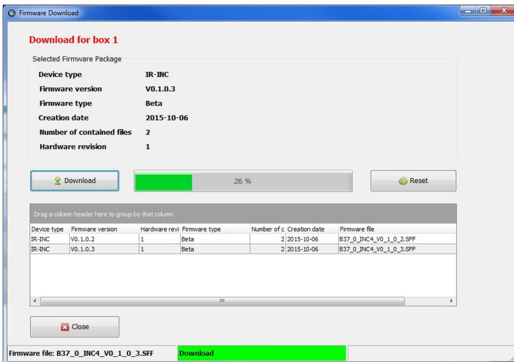
If only one firmware package for the box type has been detected, the Firmware Download window automatically selects the package. The download can be started by pressing the "Download" button:
