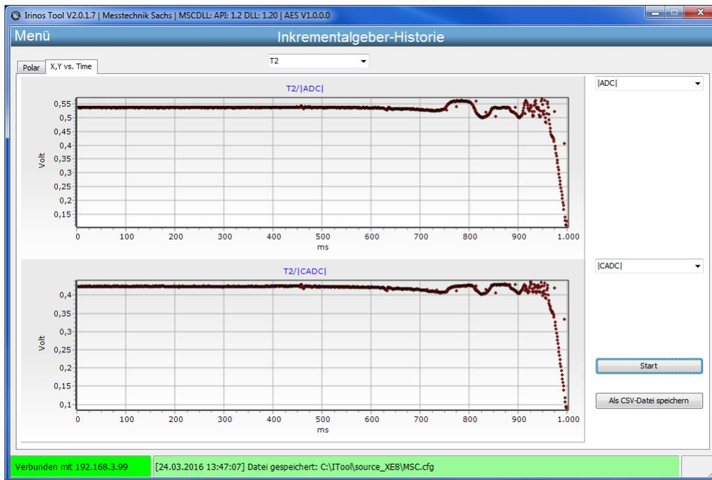
Two vertically arranged diagrams allow for a time-based correlation of different values. Via selection menus besides the diagrams, the values to be displayed can be selected:
