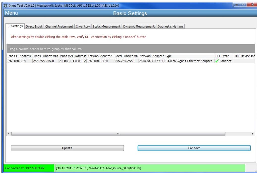
*Connection Test via the MscDll*
