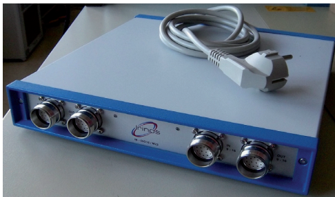
I/O-Box for I/O-Bus with integrated power supply
